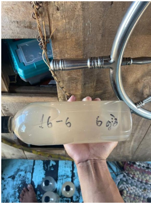
Figure 3.5. Suspended Sediment samples are collected and kept in a plastic bottle at the offshore station.
