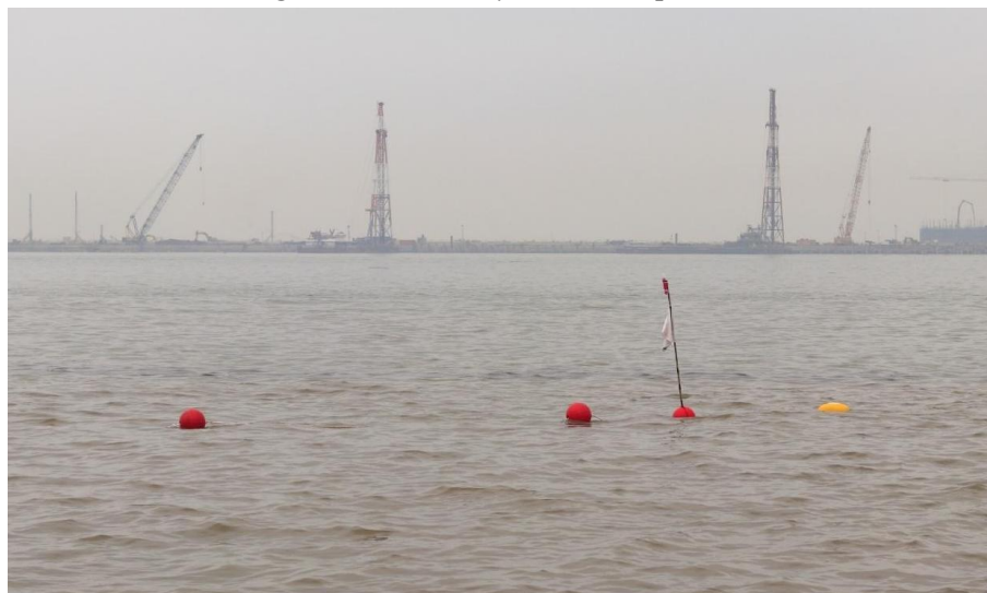
Figure 1.7. The wave buoy system has been installed. Two red balls on the left side are the in-line floating connected with easy-spot objects (flags and lights). The yellow spot on the right is the wave buoy. This system can work up to 12 months under normal conditions.
