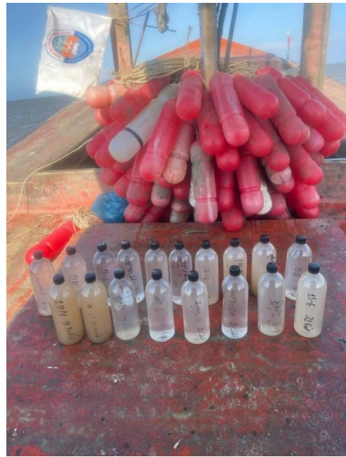
Figure 3.5. Suspended Sediment samples are collected and kept in a plastic bottle at the offshore station.
