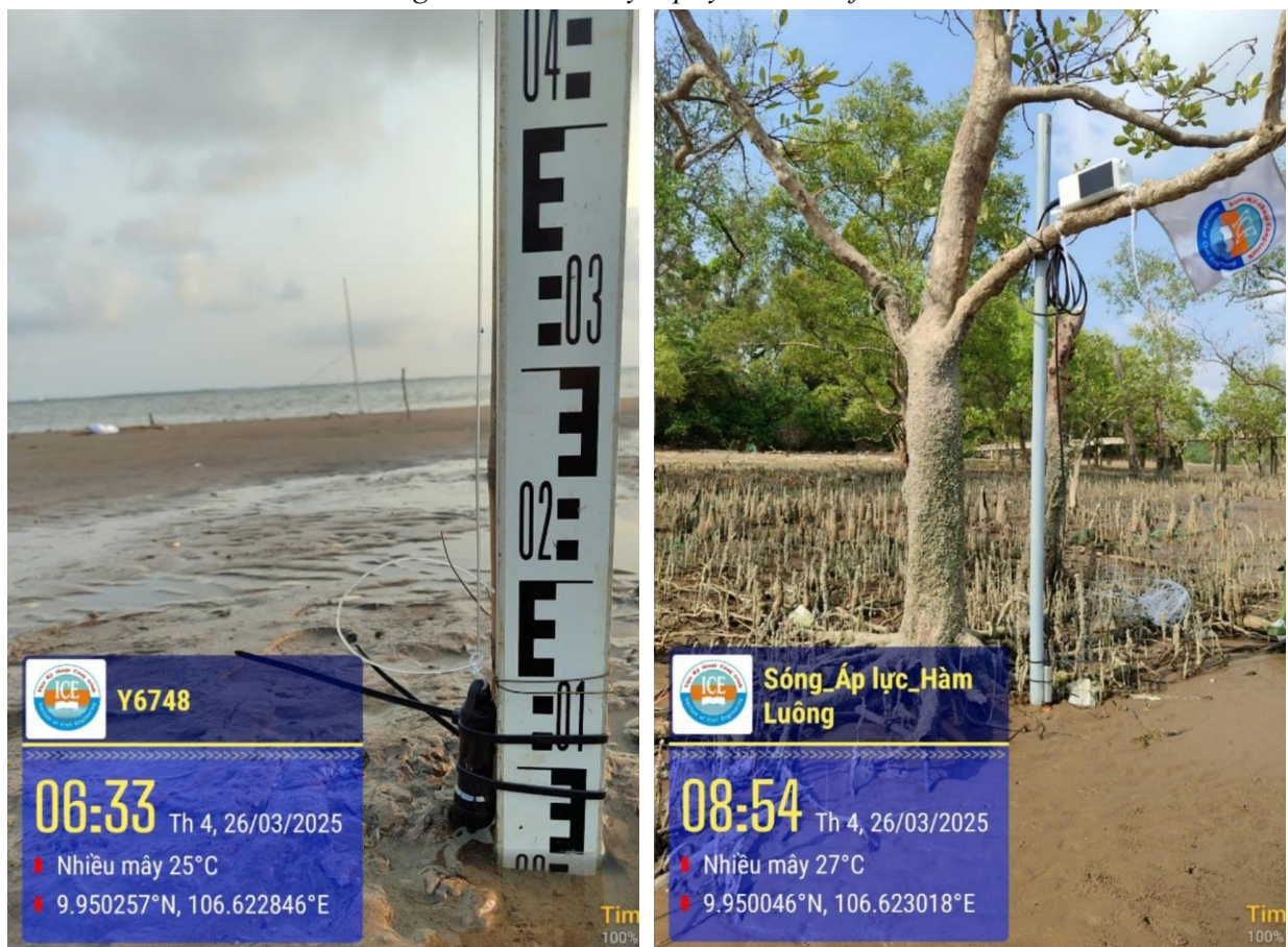
Figure 2.3. Wave gauge and Divers deployment. The diver in the left panel measured the water depth/level at the seaward location while the one in the right panel did the same job at the mangrove edge.
