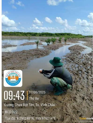
Figure 3.5. Suspended Sediment samples are collected and kept in a plastic bottle at the offshore station.
