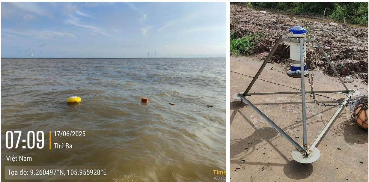
Figure 3.2. Wave buoy (left) and Sentinel-V20-ADCP (right panel)
